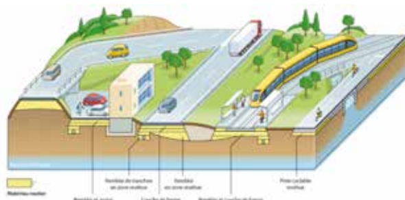
Figure 18 : Usages routiers "type 1" des mâchefers
